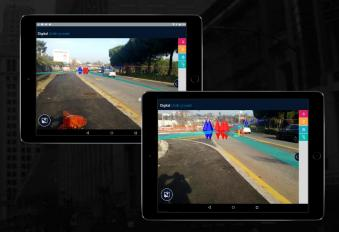
Displays **spatially accurate 3D utility data** using mobile device sensors such as GPS, magnetometer, accelerometer and gyroscope
