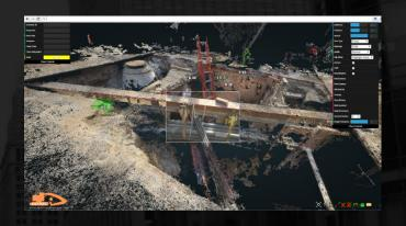
Scanning technology to transform regular video or **photos into point clouds** and then transforming **point clouds into 3D objects**
